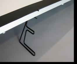
The optional available set up support allows an easy mounting of the legs. By means of the 4 round bar holders the wings screws can be bolted by one person only without holding the frame and leg in position.
