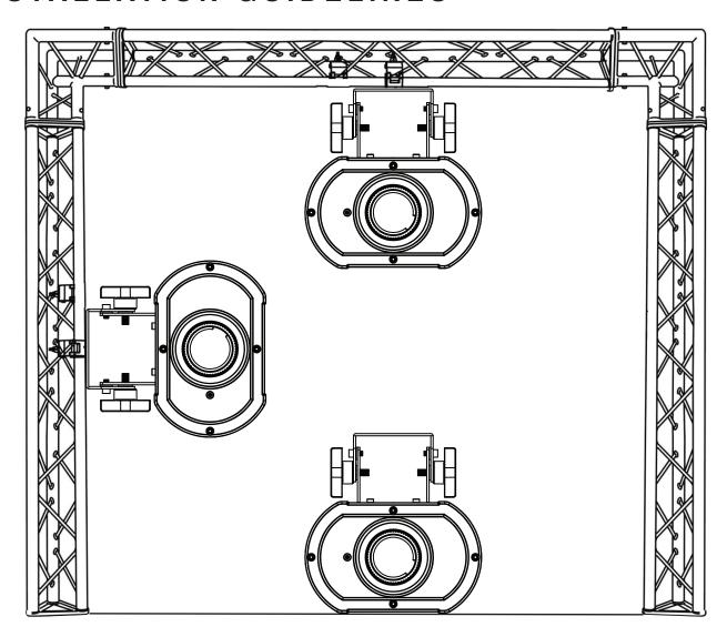
The unit is fully operational in three different mounting positions: hanging upside-down from the ceiling or trussing, sideways on trussing, or set on a flat level surface. Be sure this fixture is kept at least 2m (6.5 ft) away from any flammable materials (decorations, etc). Always use and install a safety cable (not included) as a safety measure to prevent accidental damage and/or injury in the event the clamp fails. Never use the carrying handles for secondary attachment.
