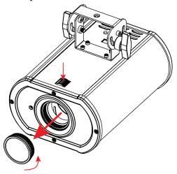
2. Remove the retainer clip from the lens assembly, then remove the lens itself.
