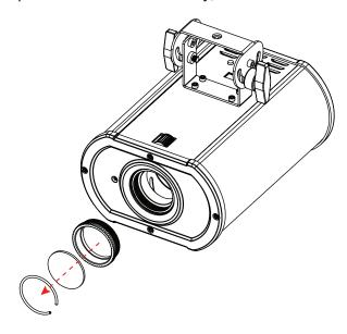
3. Replace the lens and reinstall the retainer clip to secure the lens in place. Reinstall the lens assembly in the unit by inserting the lens assembly back into the front of the unit and rotating the lens assembly clockwise while holding down the focus adjustment knob.
