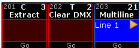
X-keys as executor with assigned macros
