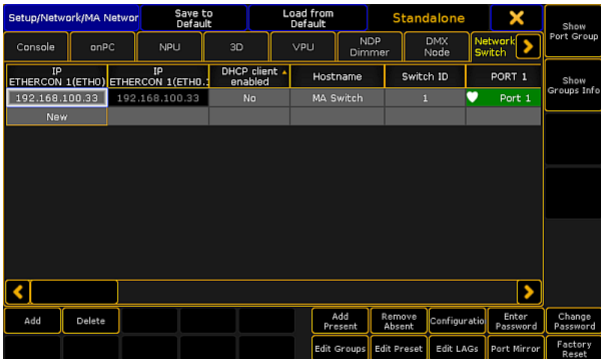
MA Network Configuration - Network Switch
